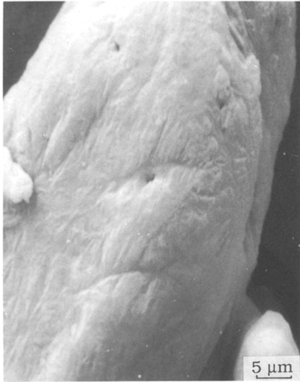
Figure 4 Topography of a powder particle showing an uneven surface.
